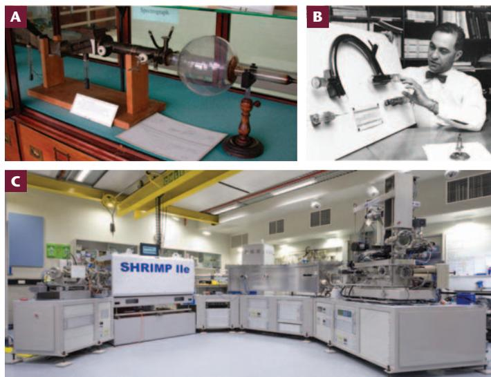
**FIGURE 2** (A) Aston’s third mass spectrograph, used for Pb isotope analysis (COURTESY OF CAMBRIDGE PHYSICS OUTREACH); (B) Alfred Nier with the flight tube of his 180° mass spectrometer, used to measure the isotopic composition of uranium (UNIVERSITY OF MINNESOTA, COURTESY OF AIP EMILIO SEGRE VISUAL ARCHIVES); (C) for comparison, a modern SHRIMP IIe SIMS instrument (SOURCE: GEOSCIENCE AUSTRALIA)
