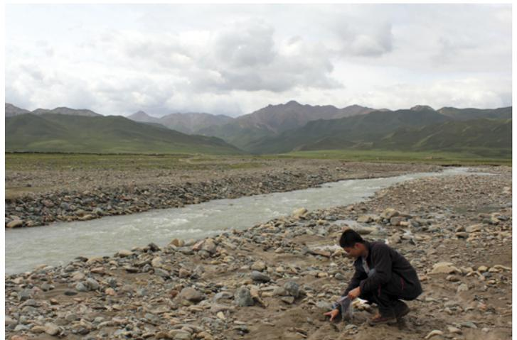
**FIGURE 2** Sampling river sand for cosmogenic nuclide determination in the Qilian Shan, northern China. A single sample of 10–100 g of quartz can yield the spatially averaged erosion rate of the sediment-contributing area upstream. PHOTO COURTESY OF KAI HU
